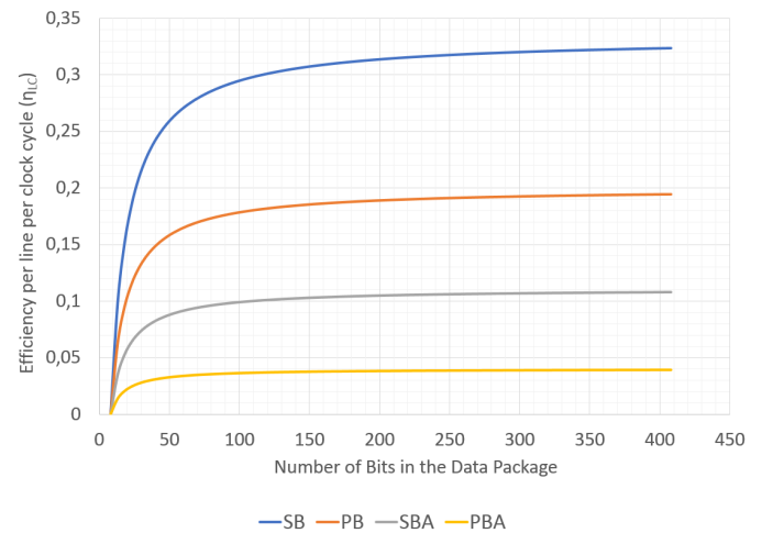
Fig. 3. Comparison of \eta_{LC} for each bus, assuming M = 4 . Observe how \eta_{LC} converges to 1/(1 + 2 \cdot M) for a SBA bus implementation and to 1/4 for a SB , as the number of bits in the flit increase; in the cases of the parallel buses, \eta_{LC} for a PBA converges to 1/(5 \cdot (1 + M)) and to 1/5 for a PB .
